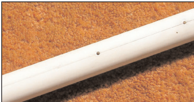
Remnants of the “chalk line” – drawn by hand using a pencil and straight edge – can be seen along the antenna’s PVC boom, where pass-through holes for the elements were drilled.
