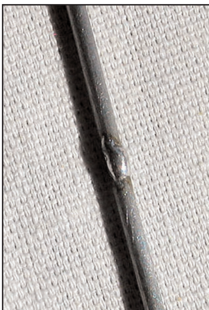
A small dollop of solder added to directors D1-4 and the reflector (REF) prevents the elements from sliding through holes drilled in the boom.
