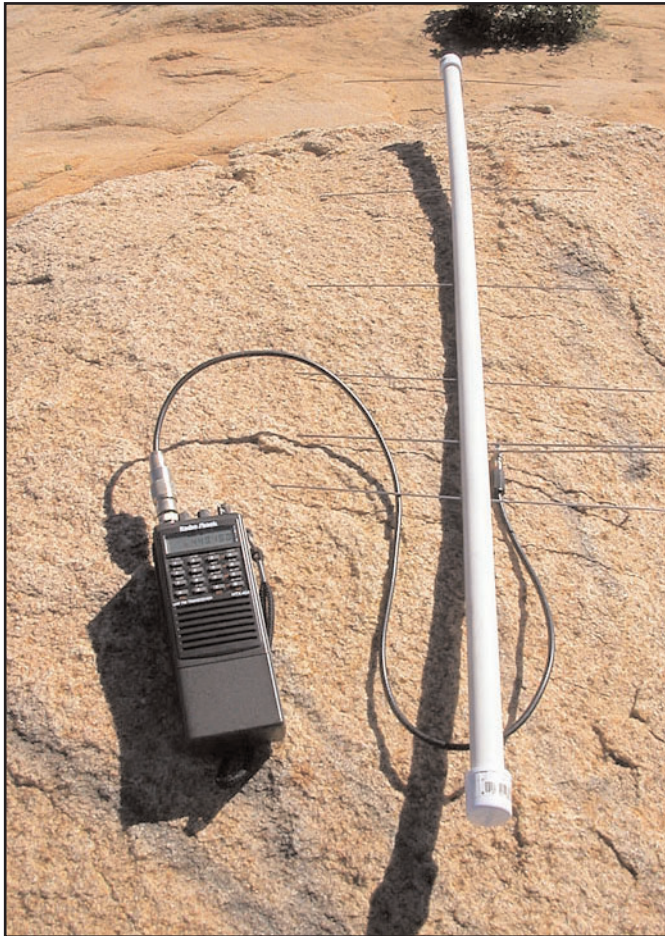
A vintage Radio Shack HTX-404 70cm FM transceiver is connected to the antenna's driven element using a standard RCA plug and jack.
