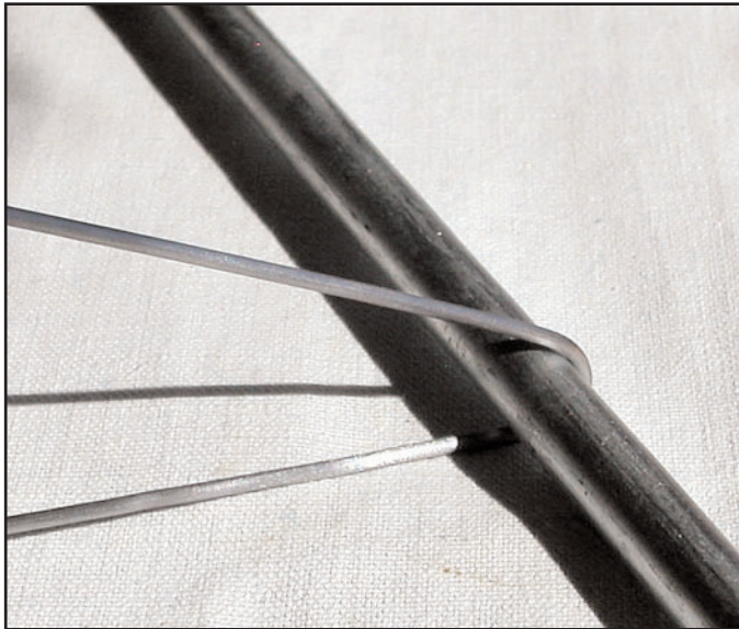
A half-inch diameter metal rod was used as a “former” at KI6SN to provide the hairpin bend in the driven element, as illustrated in Figure 1.
