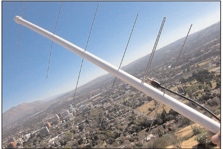
A lightweight 6-element 440 MHz FM beam antenna that's inexpensive and a snap to make performed nicely from the top of Mount Rubidoux in Riverside, California, on ARRL January VHF Sweepstakes weekend.
